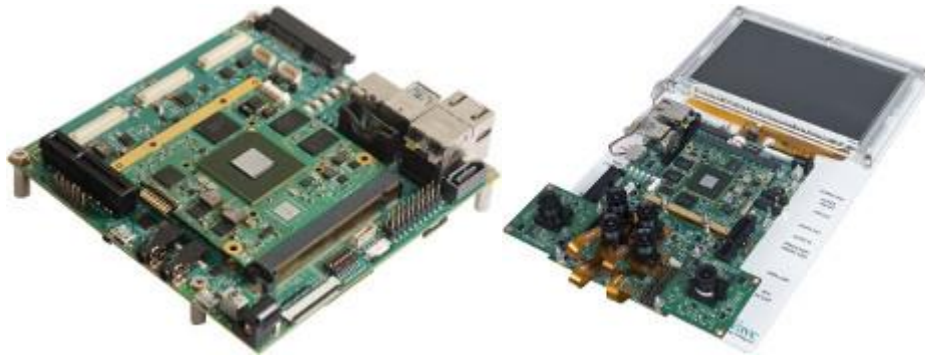
RZ/G1H dev kit carrier board (left) and full kit with 7-inch display and camera daughter board (click images to enlarge)
