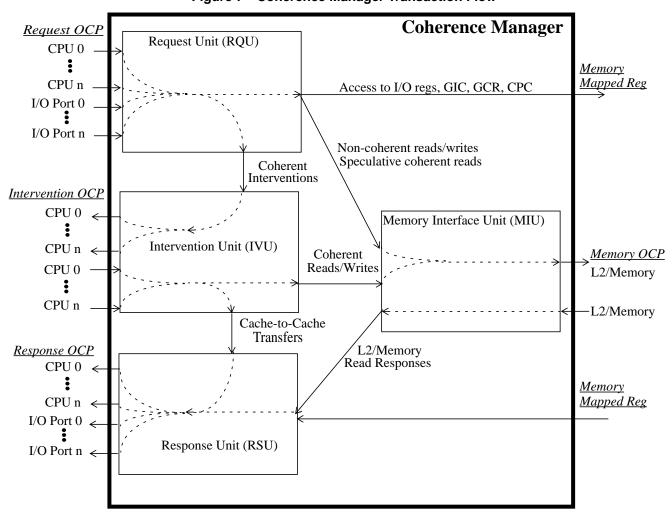
Figure 7 Coherence Manager Transaction Flow
