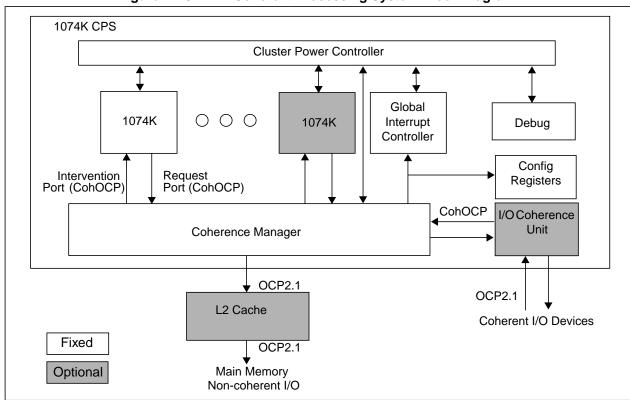
Figure 1 1074K<sup>™</sup> Coherent Processing System Block Diagram
